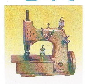
Single Needle, Plain Feed, Flat Bed, Double Thread Chain Stitch Machine for seaming and hemming openings of very heavy weight fabric such as jute or PP/PE woven cloth bags. Extra heavy duty machine for sewing very thick material with chain stitch. Single thread chain stitch is available by replacing some parts.
